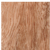
WA Spotted Gum Timber Code SPG Eucalyptus Henryi Grown in Australia Density 950 kg/m3 dry
