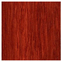
WA Jarrah Timber Code JAR Eucalyptus Marginata Grown in Australia Density 820 kg/m3 dry
