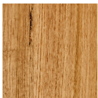
Tasmanian Oak Timber Code TOA Eucalyptus Obliqua Grown in Australia Density 780 kg/m3 dry
